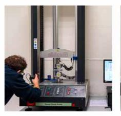
Tests for measuring the tensile strength and stretching of insulators and sheaths
